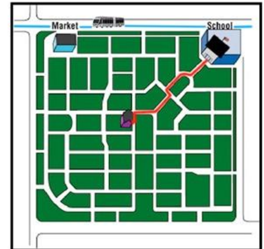
Figure 16 Congress for New Urbanism images shows the increase in distance to local facilities in a cul-de-sac and distributor model
