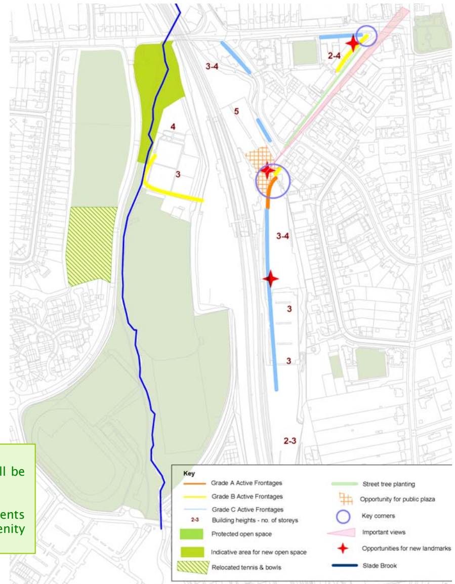
Figure STQ.4: Frontages, building heights & spatial requirements
