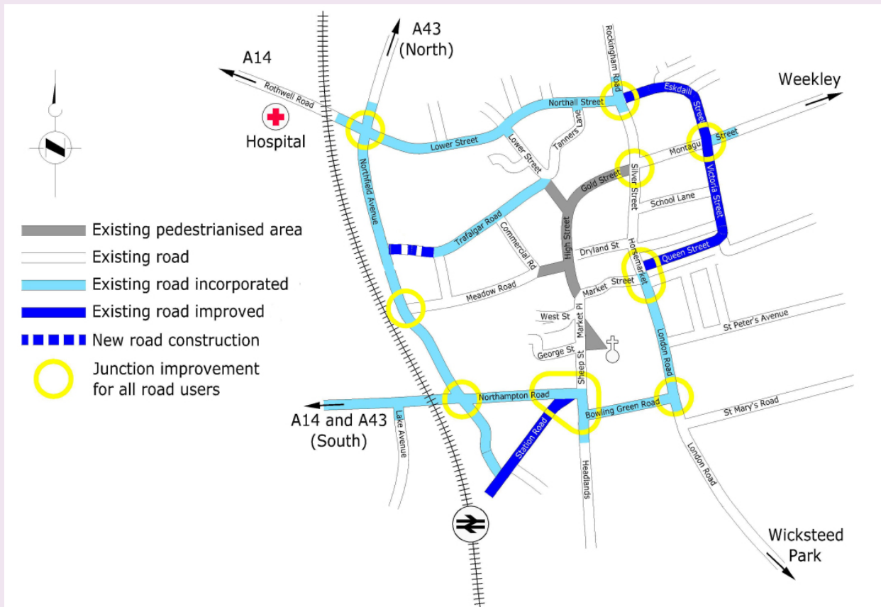
Figure 3.2 Road network and junction improvements
