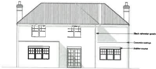
SOUTH WEST ELEVATION
