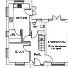
GROUND FLOOR PLAN TYPE D/1 (PLOTS 4 & 49) House complies with Space Standards
