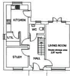
GROUND FLOOR PLAN TYPE D (PLOTS 20 & 24) House complies with Space Standards
