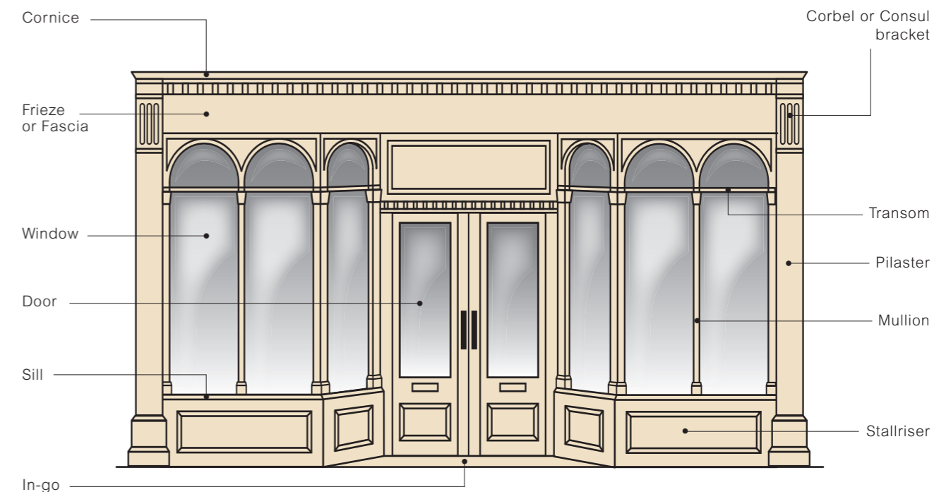
The illustration above identifies some key features of a traditional shopfront design
